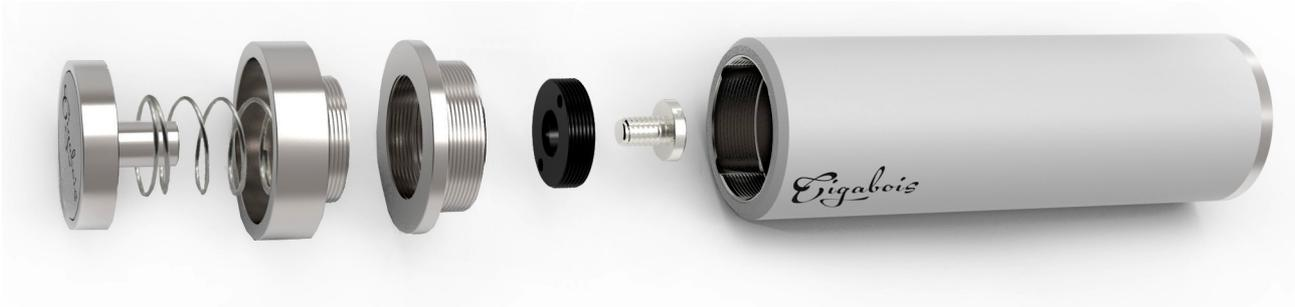
The Phileas mechanical mod uses "hybrid" connection system: the battery is in direct contact with the central pin of the atomizer. For this reason and in order to avoid any short circuit, it is absolutely necessary for the central pin of the atomizer to stick out at least 0.4 mm from the bottom of the 510 connector of the atomizer. Battery used must be in perfect condition, without any defects, cracks on the wrapper or deformed/dented poles.
